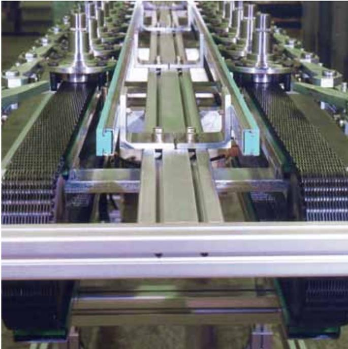
Inverted tooth chains differ considerably in their design from other steel sprocket chains. The plates form a positive locking contact with the wheels of the chain, at the same time taking on the tensile force. In this way inverted tooth chains transmit higher torques and power in confined installation spaces. The main design characteristic is the cradle-type joint made of two profile trunnions. This joint design
